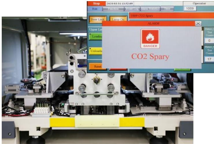
Clamping System and Fire Detection Sensor
