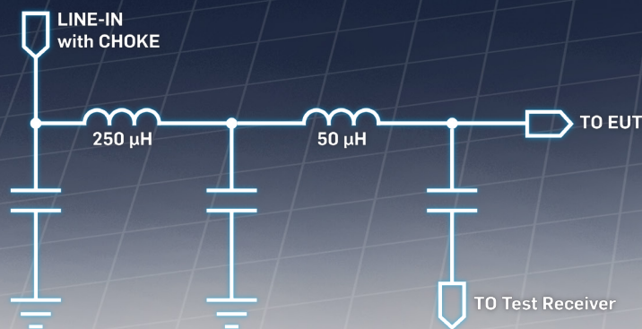
L3-100 equivalent circuit
