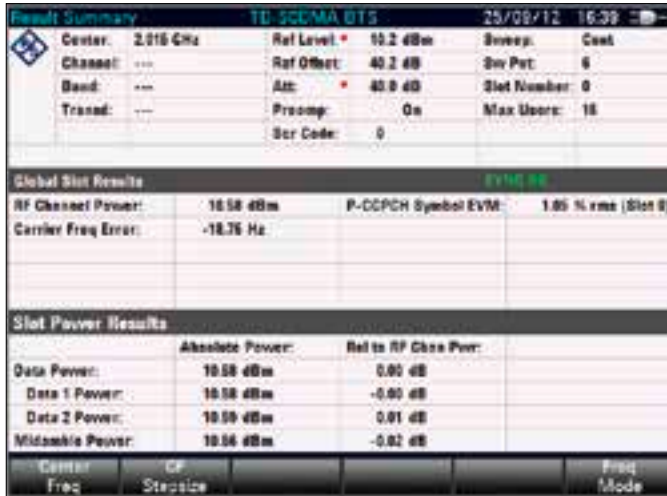
Analysis of TD-SCDMA transmit signals.
