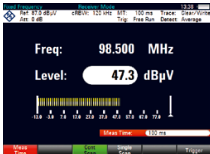
EMC precompliance measurement at a fixed frequency with adjustable measurement time.
