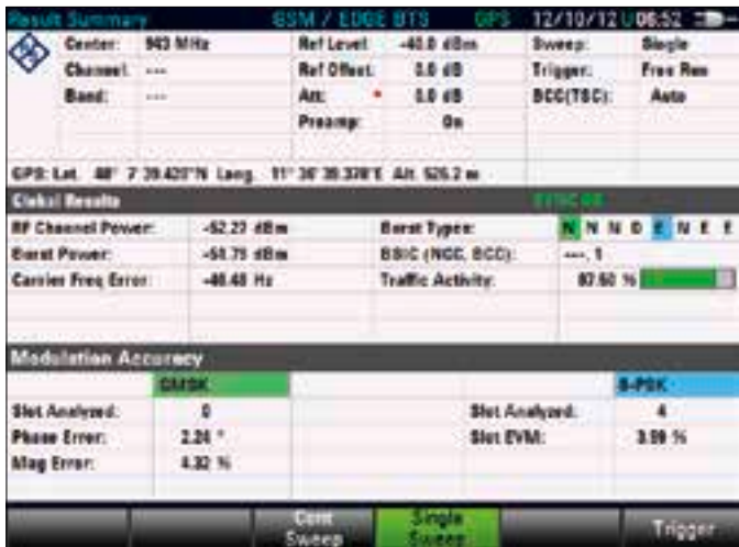
Analysis of GSM/GPRS/EDGE transmit signals.
