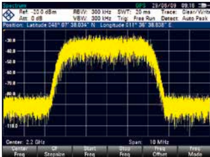
Display of the current position with the R&S HA-Z240 GPS receiver connected.
