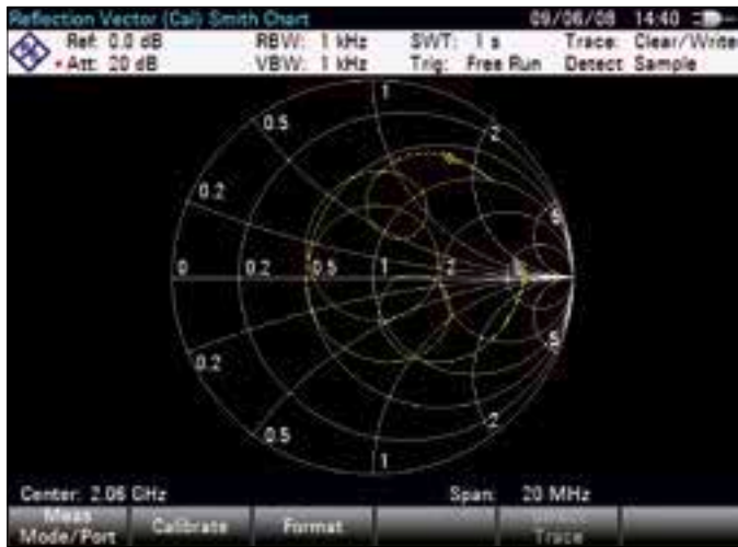
Vector network analysis: measurement with Smith chart.
