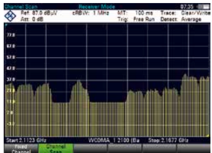
Channel scan of a 3GPP WCDMA frequency band.
