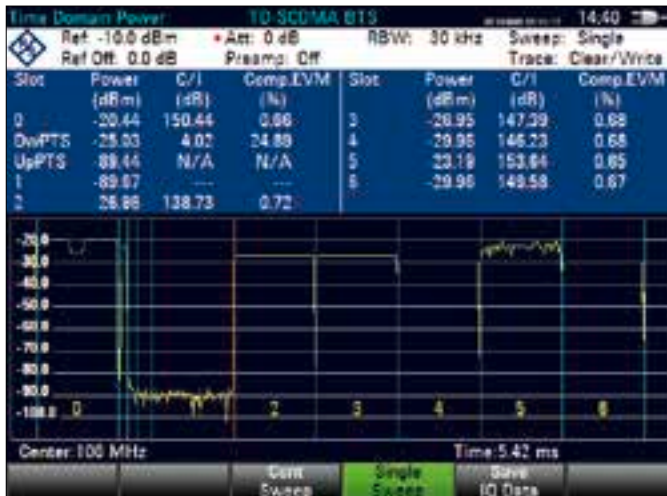
TD-SCDMA time domain display is available with the R&S®FSH-K48E option.
