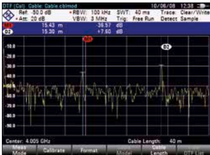
Distance-to-fault measurements (DTF).
